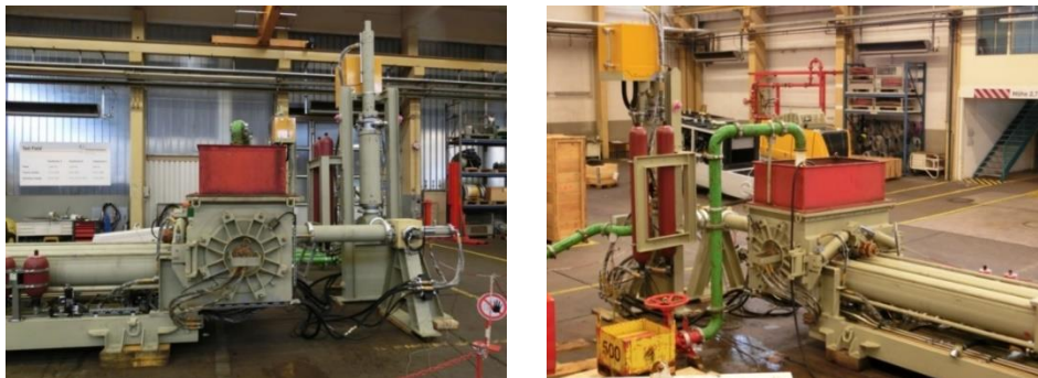
Figure 8: Hydraulic Driven S- Tube Pump with Hydraulic Pulsation Dampening System
